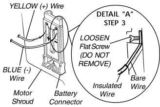
FIGURE 5 - REMOVING THE BATTERY CONNECTOR
